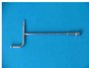
T-wrench ( for screwing bolts of outer case )
