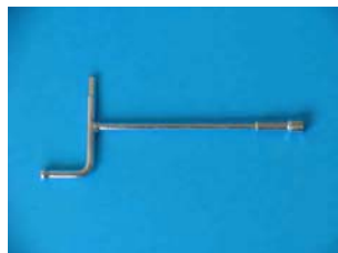
T-wrench ( for screwing bolts of outer case )
